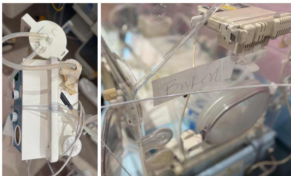
Fig. 21. The consequences of poor equipment maintenance are obvious: improvised repair of suction device (left), broken incubator (right).
