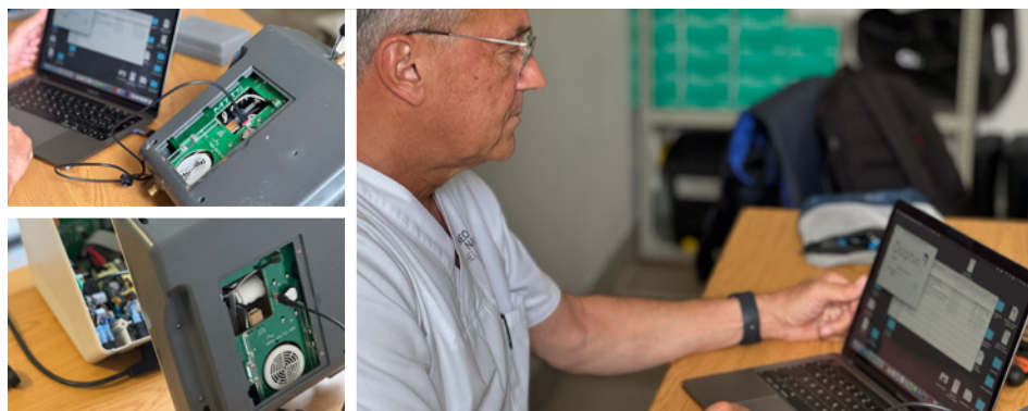
Fig. 6. Installation of new ultrasonic oxygen sensors (part II): the process is completed with a software update.
