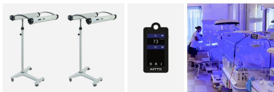
Fig. 4. MTTS Colibri® phototherapy unit (left) and MTTS light meter (middle): the latter allows to measure light intensity (example shown: 31 \mu\text{W}/\text{cm}^2/\text{nm} from above, 42 \mu\text{W}/\text{cm}^2/\text{nm} from below (e.g., bilirubin blanket), total 73 \mu\text{W}/\text{cm}^2/\text{nm} ) and determine whether the unit can still be used for patients (right).
