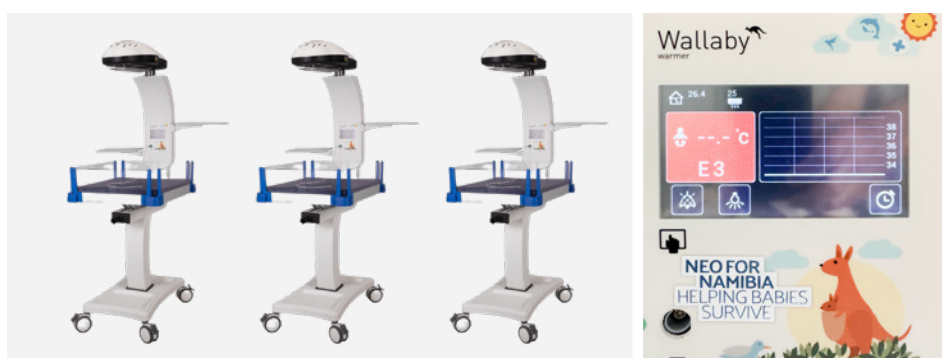
Fig. 3. MTTS Wallaby® open warmers: three out of eight units donated will need new heating elements as indicated by “E3” on the display; in another unit “E1” indicates that a software update is needed.
