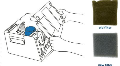
Fig. 17. The Pumani<sup>®</sup> bubbleCPAP device (left) has an integrated pump (blue) to generate air flow; air enters the device on the bottom, and dust is eliminated by simple filters (right) before it is directed into the machine's internal tubing system.
